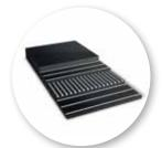
The Translev M has a **full steel carcass design**. Steel cords in longitudinal direction provide high nominal belt strength at low elongation, as well as two layers of steel wefts in cross direction. This construction provides the highest bolt pull-out values combined with the highest possible puncture resistance.
